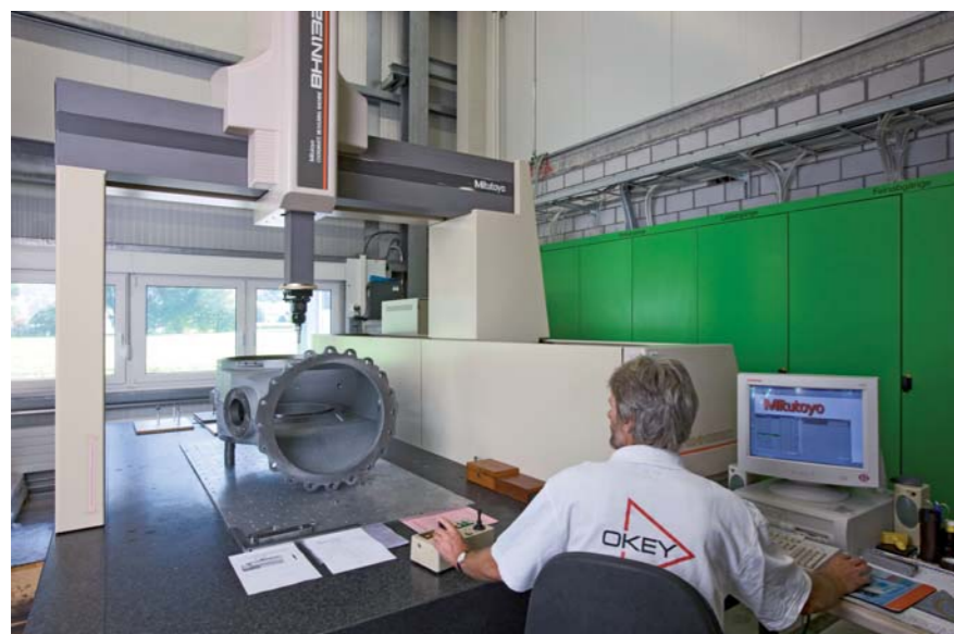
3-D-Messmaschine Mitutoyo BN 1320
